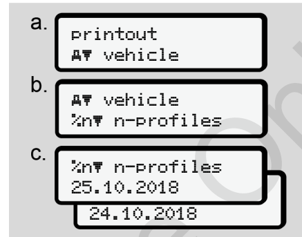
Fig. 97: Menu sequence printout - speed profiles
